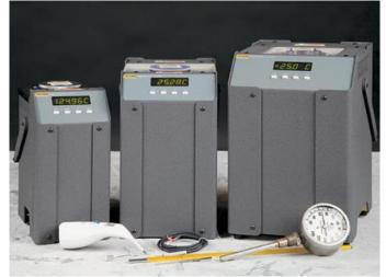
Drywells / Metrology Wells use a solid metal block as the controlled temperature volume
